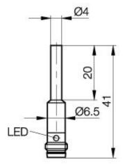
Inductive Sensors BES 516-3008-E5-C-S49 D4 x 41 normally-open Sn=0,8mm shielded
